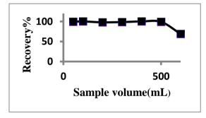
**Figure 4.** Effect of sample volume on recovery of lead Conditions: Pb, 5.0  $\mu$ g;; flow rate, 3.0 mL min<sup>-1</sup>; sorbent, 50.0 mg; elution solution, 5.0 mL 0.5 mol L<sup>-1</sup> HNO<sub>3</sub>
