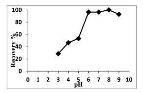
Figure 3. Effect of pH on recovery of lead
