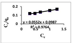
Figure 5. Langmuir isotherm for lead
