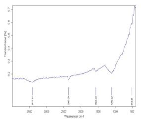
Figure 1. IR spectrum of bare activated carbon
