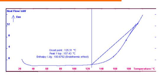
Figure 7. Oleic acid and 1000 ppm zingiber officinale essential oil oxidation stability thermogram
