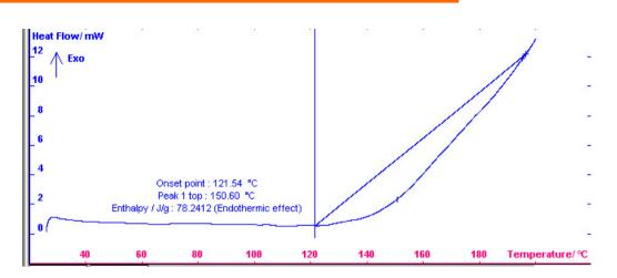
Figure 4. Oleic acid and 250 ppm zingiber officinale essential oil oxidation stability thermogram
