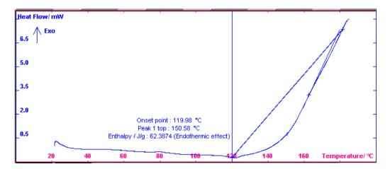
Figure 3. Oleic acid oxidation stability thermogram
