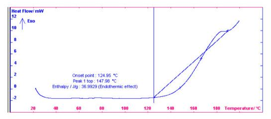
Figure 6. Oleic acid and 750 ppm zingiber officinale essential oil oxidation stability thermogram
