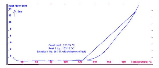
Figure 5. Oleic acid and 500 ppm zingiber officinale essential oil oxidation stability thermogram
