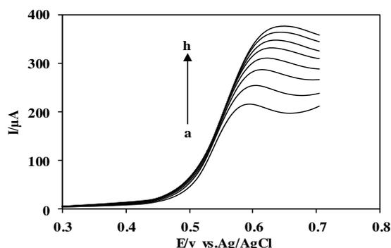
**Figure 5.** Pseudo-steady state polarization curves of Ni/Al LDH-SGD-CC electrode obtained from (a) to (h) 0.02, 0.03, 0.04, 0.05, 0.06, 0.07, 0.08 and 0.09M acetaldehyde, respectively.
