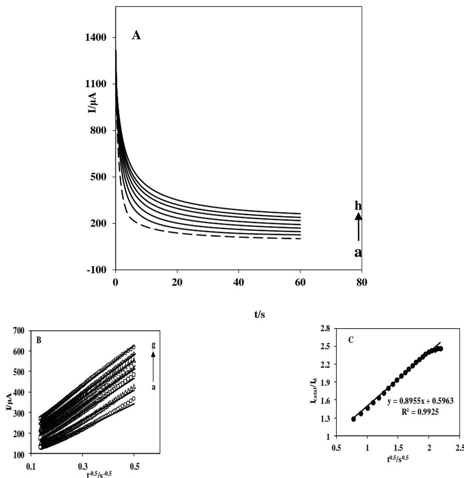
**Figure 4.** (A) Chronoamperograms of Ni/Al LDH-SGD-CC electrode in 0.1 M NaOH containing different concentrations of acetaldehyde: 0.0, 0.01, 0.02, 0.03, 0.04, 0.05, 0.06 and 0.07 M acetaldehyde, from (a) to (h), respectively. Potential steps were 0.65 and 0.0 V, respectively. (B) Dependency of transient current on  $t^{-1/2}$ . (C) Dependency of  $I_{\text{cat}}/I_d$  on  $t^{1/2}$  derived from CAs of (a) and (h) in panel (A).
