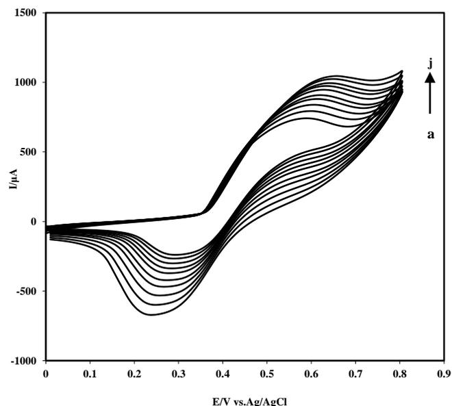
**Figure 2.** CVs of different concentrations of acetaldehyde at Ni/Al LDH-SGD-CC electrode in 0.1 M NaOH at a scan rate of  $50 \text{ mV s}^{-1}$ . Concentrations of acetaldehyde from (a) to (j) are 0.01, 0.02, 0.03, 0.04, 0.05, 0.06, 0.07, 0.08, 0.09 and 0.1M, respectively.
