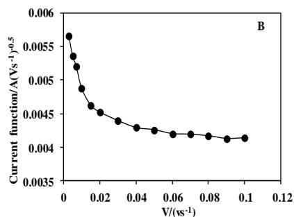
**Figure 3.** (A) Cyclic voltammograms of Ni/Al LDH-SGD-CC electrode in 0.1M NaOH containing 0.05 M of acetaldehyde at various potential scan rates (from inner to outer) 3-100 mVs<sup>-1</sup>. Variation of the catalytic current with the square root of sweep rate (inset). (B) Current function vs. V for 0.1M NaOH solution in the presence of 0.05M acetaldehyde.
