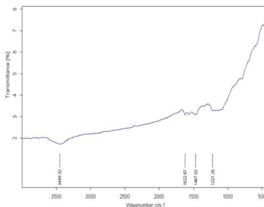
Figure 2. IR spectrum of modified activated carbon
