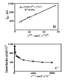
Figure 6 a. CVs of the Ni/SDS/CPE in the presence of 0.1 M methanol at different scan rates: a 10, b 20, c 50, d 80, e 100, f 200, g 400, h 600 and i 800 mV s<sup>-1</sup>, respectively, b The dependency of  $I_p$  on <sup>1/2</sup> and c variations of an anodic current function vs.
