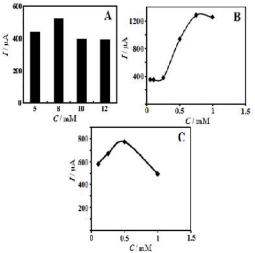
**Figure 7.** Effect of a SDS concentration, b nickel concentration and c sodium hydroxide concentration on oxidation currents of 0.1 M methanol at the surface of Ni/SDS/CPE, v = 20 mV s<sup>-1</sup>
