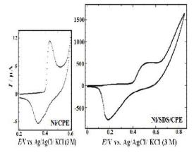
Figure 2. CVs of Ni/CPE and Ni/SDS/CPE in 0.1 M NaOH solution,  $v = 20 \text{ mV s}^{-1}$
