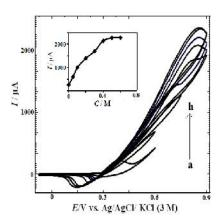
**Figure 8.** CVs of the Ni/SDS/CPE in 0.5 M NaOH solution with different concentrations of methanol *a* 0, *b* 0.05, *c* 0.1, *d* 0.2, *e* 0.3, *f* 0.4, *g* 0.5, and *h* 0.6 M, v = 20 mV s<sup>-1</sup>, Inset: Plot of  $I_{pa}$  vs. methanol concentration
