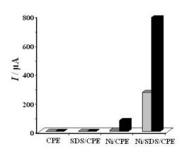
**Figure 5.** Comparison of anodic currents for various electrodes: in 0.1 M NaOH solution in the absence (gray bar), and presence (black bar) of 0.1 M methanol. Scan rate:  $20 \text{ mV s}^{-1}$
