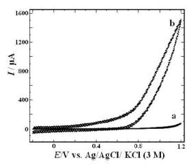
Figure 1. CVs of (a) CPE and (b) SDS/CPE in 0.1 M NaOH solution,  $v = 50 \text{ mV s}^{-1}$
