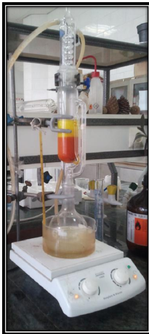
Figure 1. The soxhlet extractor
