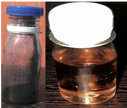
**Figure 2.** Images of synthesized GO powder and solution
