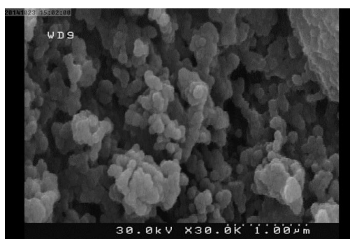
Figure 4. SEM images of magnetically recycled ZnCrFeO_4 after three runs
