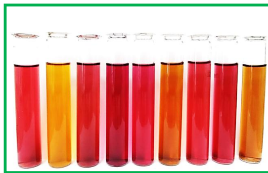
Figure 5. Color change of 5.0 \times 10^{-4} M solution of 8b in presence of various anions. From left to right: None, \text{CN}^- , \text{Cl}^- , \text{Br}^- , \text{I}^- , \text{OAc}^- , \text{H}_2\text{PO}_4^- , \text{NO}_3^- , \text{NO}_2^-
