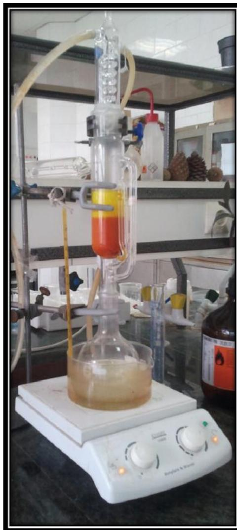
**Figure 1.** The soxhlet extractor
