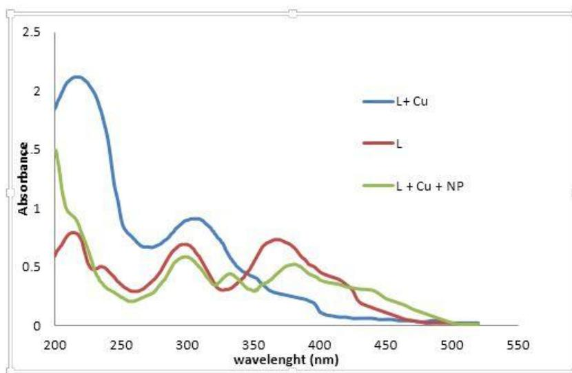
**Figure 2.** UV-Vis absorption spectra of EAMT, EAMT-Cu and EAMT-GNP-Cu.
