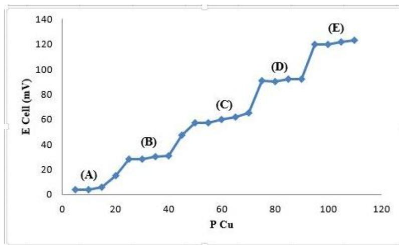
**Figure 5.** Dynamic response of the AMT-GNP carbon paste electrode for step changes in  $\text{Cu}^{2+}$  concentration: (A)  $10^{-7}$  M, (B)  $10^{-6}$  M, (C)  $10^{-5}$  M, (D)  $10^{-4}$  M, and (E)  $10^{-3}$  M.
