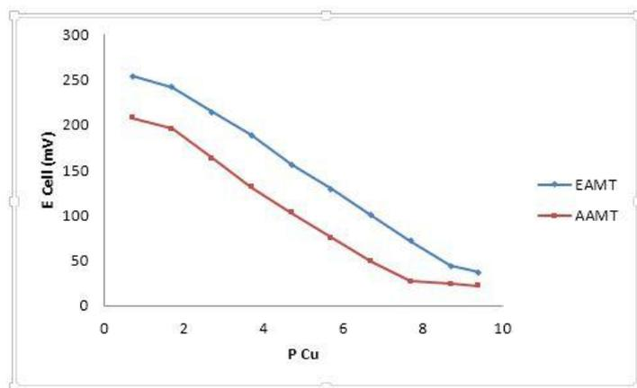
**Figure 3.** Calibration curves for Cu (II)-carbon paste electrode based on EAMT and AAMT at pH~ 4.0.
