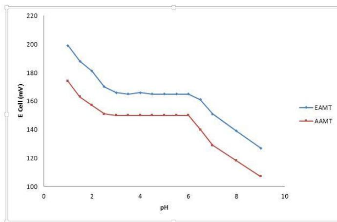
**Figure 4.** The pH effect of the test solution on the potential response of the proposed  $Cu^{2+}$  carbon paste electrodes.
