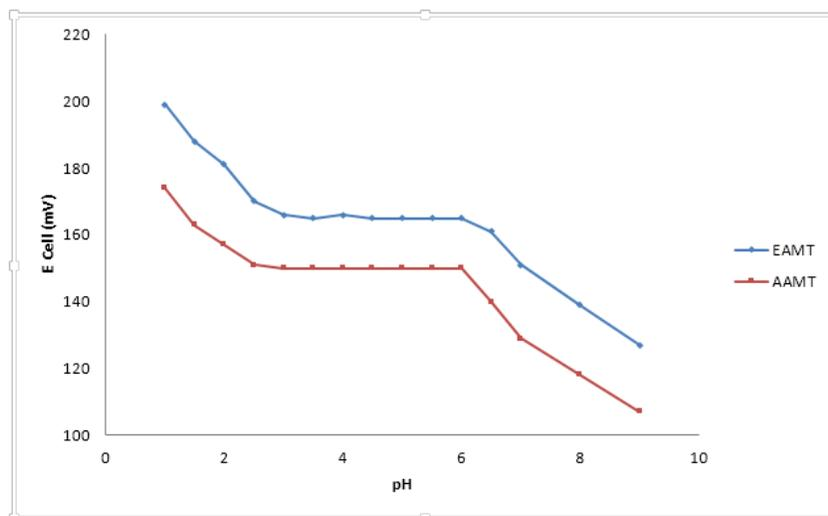
**Figure 6.** Potential titration curves of 25.0mL  $1.0 \times 10^{-4}$ M Cu ( $\text{NO}_3$ )<sub>2</sub> solution with  $1.0 \times 10^{-2}$ M of EDTA.
