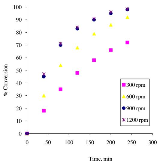
**Figure 1.** Effect of various stirring speeds on the conversion: 0.04 mol of disodium salt of 1,3-dihydroxybenzene, 0.01 mol of propargyl bromide, 0.2 g of biphenyl, 50 mL of toluene, 0.0015 mol of TBAB, 50 °C
