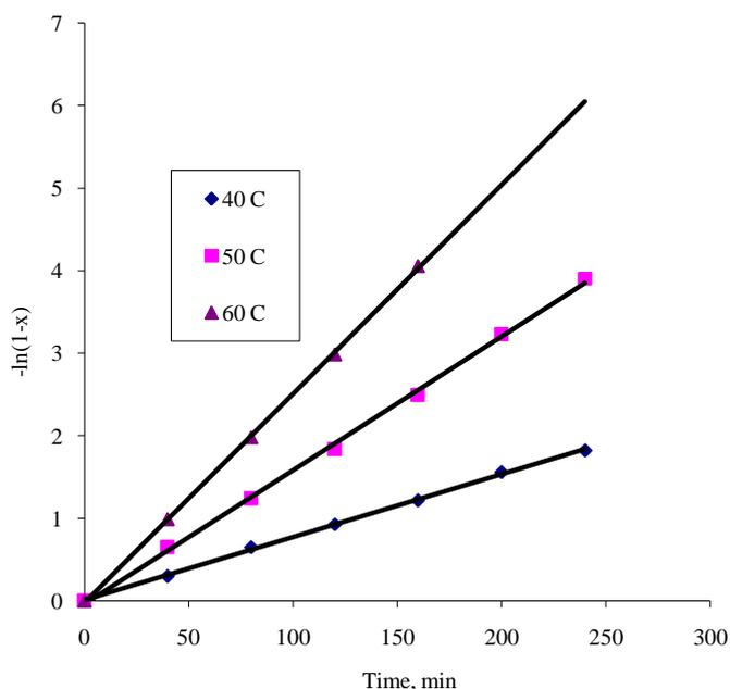
**Figure 2.** Effect of reaction temperatures on the conversion of propargyl bromide. 0.04mol of disodium salt of 1,3-dihydroxybenzene, 0.01 mol of propargyl bromide, 0.2 g of biphenyl, 50 mLof toluene, 0.0015 mol of TBAB, 1200 rpm.
