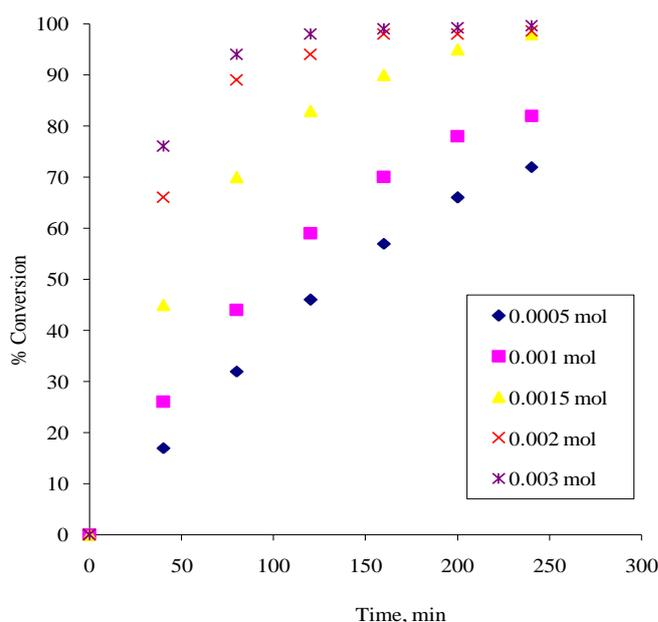
**Figure 3.** Effect of TBAB loading on the conversion of propargyl bromide: 0.04 mol of disodium salt of 1,3-dihydroxybenzene, 0.01 mol of propargyl bromide, 0.2g of biphenyl, 50 mL of toluene, 50 °C, 1200 rpm.
