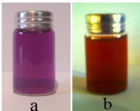
Figure 1. Photograph of (a) the Brassica oleraceae extract and (b) Ag/Brassica oleraceae emulsion after 24 h
