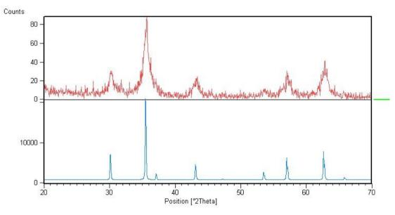
Figure 2. XRD pattern of synthesized CoFe<sub>2</sub>O<sub>4</sub>
