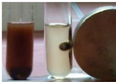
**Figure 1.** Image showing MNPs-PSA can be separated by applied magnetic field. A reaction mixture in the absence (left) or presence of a magnetic field (right)
