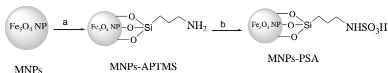
**Scheme 2.** Synthesis of supported *N*-propylsulfamic acid on magnetic nanoparticles; (a) (3-aminopropyl)-triethoxysilane (99%, 2.5 mL), ethanol/water, rt, 8 h; (b) chlorosulfuric acid (0.8 mL), dichloromethane, 2 h, rt.
