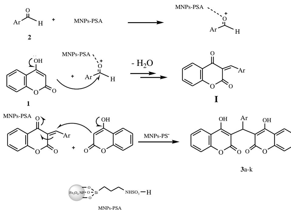
**Scheme 3.** The suggested mechanism for the formation of 3,3'-arylidene bis(4-hydroxycoumarin) catalyzed by MNPs-PSA
