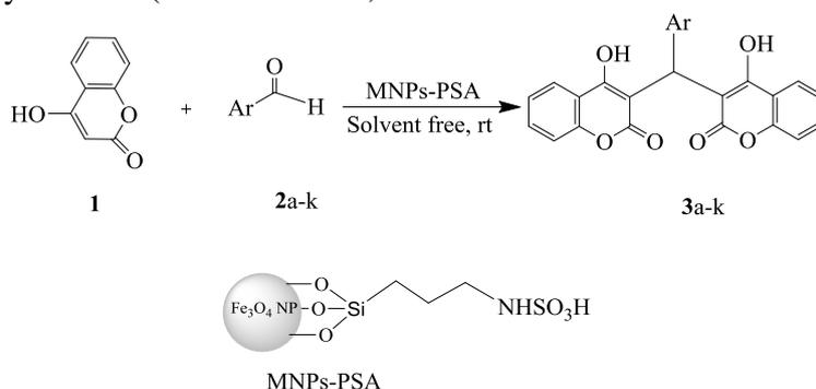
**Scheme 1.** MNPs-PSA catalyzes the preparation of 3,3'-arylidene bis(4-hydroxycoumarins)
