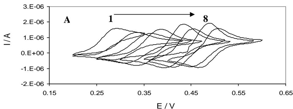
**Figure 2.** Cyclic voltammograms of activated glassy carbon electrode (AGCE) in 0.1 M phosphate buffer containing 0.2 mM Methyldopa in different pH values. The number of 8 to 1 correspond to 5.5, 5, 4.5, 4, 3, 2.5, 2, 1.5 pH. Scan rate was 25 mv / s.
