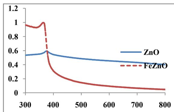
**Figure 3.** UV-Visible diffuse reflectance spectra of ZnO and FeZnO
