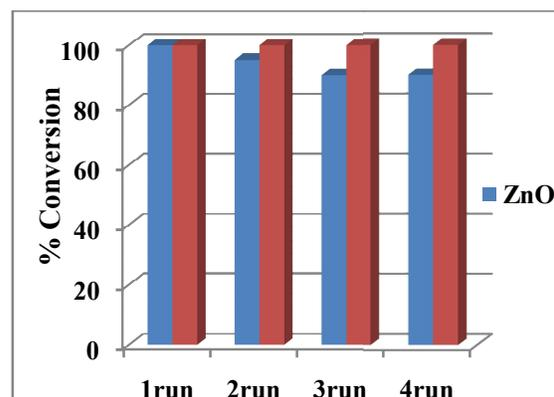
**Figure 5.** Compare the reusability of the nano ZnO and FeZnO in oxidation of benzyl alcohol after 4 times.
