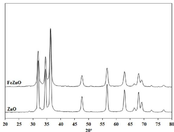
**Figure 1.** XRD data of ZnO and FeZnO
