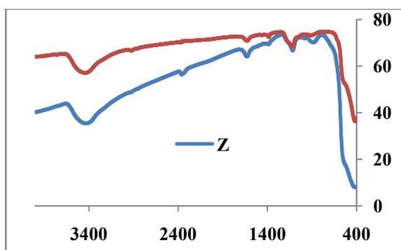
**Figure 4.** FTIR spectrum of ZnO and FeZnO
